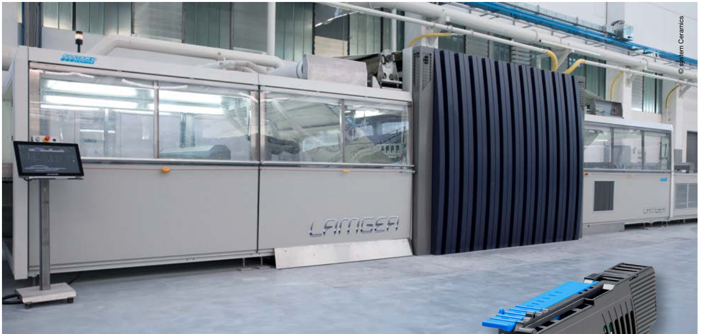
LAMGEA presses the material without a mould, so the slab is able to expand and release any internal tension.
